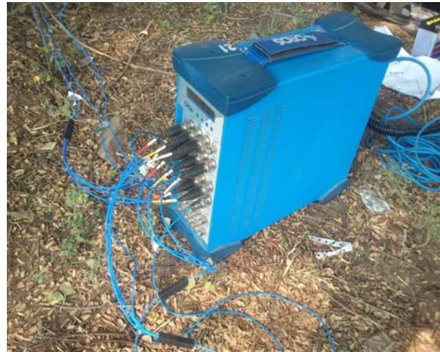
Fig-2 Sixteen Channel vibration analyser
